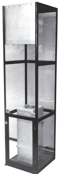
Liquid bath TZh-1-300 (as part of thermostat TR-1M) inside exhaust chamber KV-1
